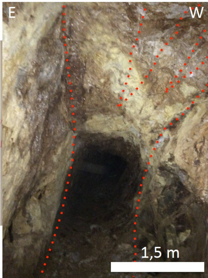
Photo 2: Another adit accessing the Guayacanes structures. An intended drill pad location is approximately 10 metres to the west of the image and is expected to intercept the veins below the current artisanal workings.
